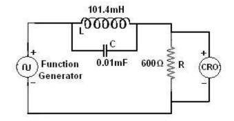
**Circuit Diagram for Parallel Resonant**
