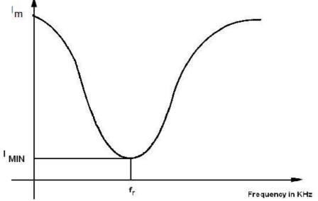
Frequency Response of Parallel Resonance Circuit
