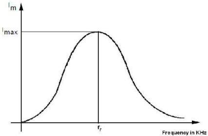
Frequency Response of Series Resonance Circuit
