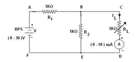
Circuit Diagram for Maximum Power Transfer Theorem <u>CALCULATION:</u>
