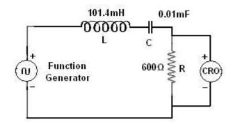
**Circuit Diagram for Series Resonant**
