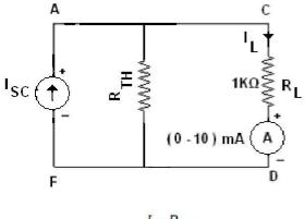
$$I_L = \frac{I_{SC} R_{TH}}{R_{TH} + R_L}$$
